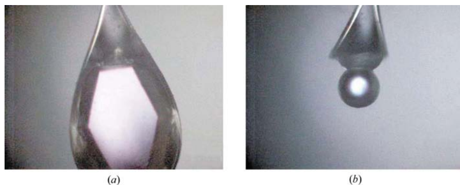
Figure 4 Example of a laser-processed protein crystal. A lysozyme crystal frozen in the standard cryoloop (a) was laser-processed to make a spherical ball-shaped crystal (b). The diameter of the sphere is 250 µm.
